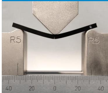
Bending test on PP-GF according to DIN EN ISO 178
