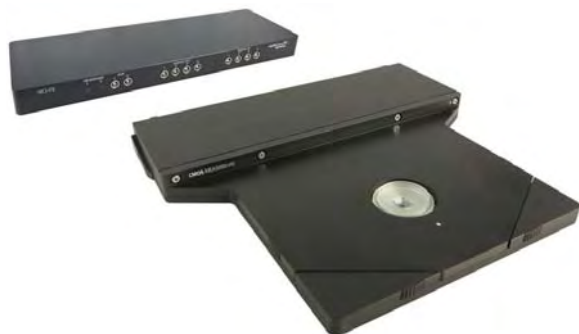
Figure 2: Chip operating unit and data acquisition system
