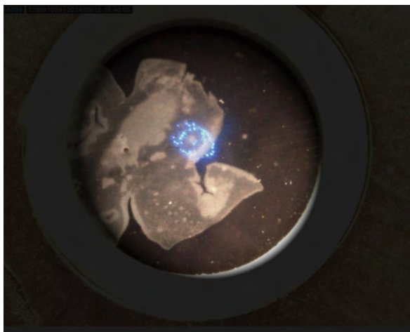
Fig.2. Photomicrograph of an isolated ChR2rd1 retina mounted on a 60-channel ITO MEA. An image projected by the LEDs is focussed onto the retina by the optical system.
