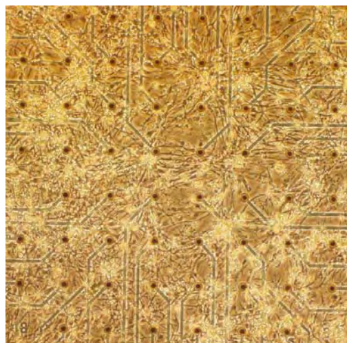
Fig. 1. Hippocampal CA1-CA3 culture (21 DIV) on a microelectrode array
