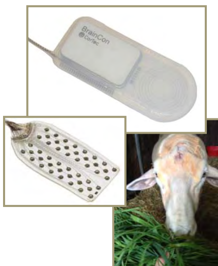
Fig. 1. Implant for EcOG-recordings with surface electrodes (provided by CorTec, Freiburg), which was tested in sheep and successfully passed the first long-term stability tests.
