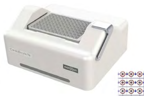
Fig. 1. Left: CardioExcyte 96 with inserted 96-Well sensor plate. Right: Sensor design of the 96-well sensor plate can be used for EFP and impedance measurements.
