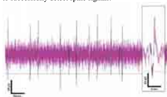
Fig. 5. Electrical recordings were performed three days after plating the cells onto the device. The AIMS was connected to a MCS measurement setup for recordings of neural electrical activities. Action potentials originating from neurites in a microchannel with amplitudes in the range of 100 \mu\text{V} and a duration of approximately 4 ms were detected.
