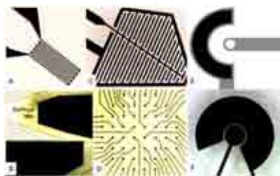
Fig. 1. Sensors of the GC 3 : A) Temperature sensor, B) Mass electrodes, C) IDES, D) Multi-electrode array (MEA), E) Circular electrode for O 2 measurement*, F) Circular electrode for pH measurement*
