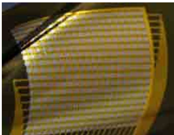
Fig. 1. High-resolution (500 \mu m spacing), flexible, active electrode array with 360 amplified and multiplexed electrodes. Only 39 wires are needed to sample from all of the 360 electrodes simultaneously.
