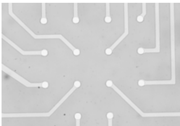
Fig. 2. MEA fabricated using photoplotting film masks. The diameter of the microelectrodes is 30 \mu\text{m} .
