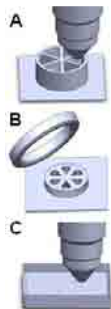
Fig. 1: Fixed versus removable dividers. (A) Solid model of the Multichannel Systems 6-well MEA and a Nikon CFI Fluor 40xW objective. The fixed divider is not compatible with high-magnification microscopy. (B) Solid model of one of our custom removable dividers and lid. (C) Solid model of MCS 6-well MEA after divider has been removed. In contrast with (A), there is ample space for high-magnification objectives. Note: MEA dimensions are 49mm x 49mm
