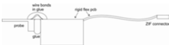
Fig. 7. Schematic view of the mechanical and electrical connection of the probe to a rigid flex board (not to scale).
