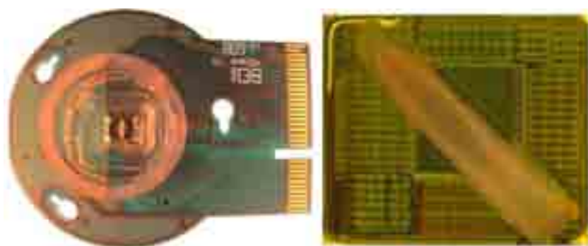
Fig. 1. HD-CMOS device and magnification of the electrode area with a root slice on top.
