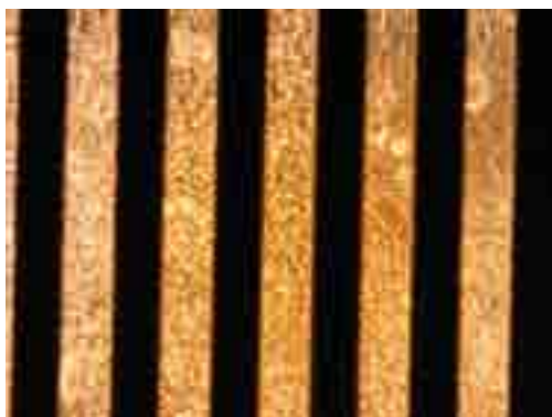
Fig. 3. Optical transmission image of confluent Caco-2 cell layer grown on the interdigitated electrode sensor (IDES). The black stripes are the optically intransparent metal electrodes of 50 \mu m width.
