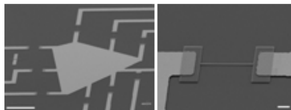
Fig. 1. Electron beam micrographs of 100 nm wide Si-NWFETs (right) integrated in a triangular array (left). The design is chosen to follow the spike propagation along a closed triangular neurons network (Fig.5). Scale bars are 40 \mu m (left) and 1 \mu m (right).
