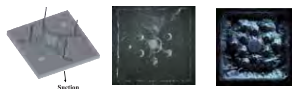
Fig. 2. A. A schematic of the planar immobilization device. An array of small pores is located in the center while larger through pores are located in the periphery for tissue pinning. B. A leech ganglion is pinned over a suspended glass membrane, demonstrating mechanical robustness of the device. C. Fabrication of an array of pores through ~20µm thick quartz is indeed possible (design from Figure 2A).
