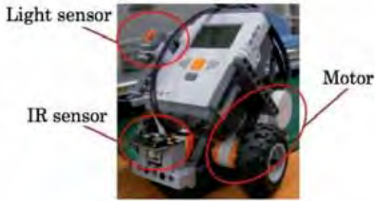
Fig. 2. Robot body constructed by Mind storm NXT kit.
