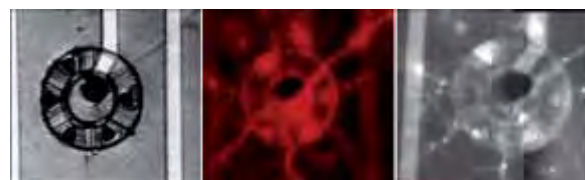
Fig. 1. Caged neuron DIC (left), voltage sensitive dye-stained (center), and NeuroCCD (right) images. The soma is adjacent to the lower-right side of the platinum black electrode.
