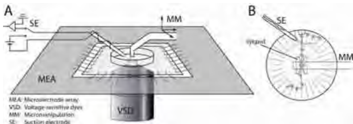
Fig. 1. The setup for combined extracellular and VSD recording. A) The setup inside the microscope. The micromanipulator (MM) is used to precisely position the ganglion over the active area. B) Top-side view of the MEA with the Sylgard carrier to keep the tenth ganglion in place. The suction electrode is placed on the sixteenth ganglion. The nerve cord is fixated to the rim of the dish caudally to ganglion 16. For clarity not all 21 ganglia are drawn. Figure not to scale.
