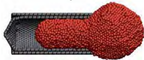
Fig. 4. Simulation of dewetting of nickel atoms (red) along the CNT wall (black)
