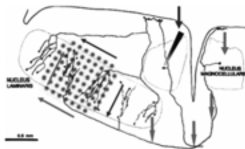
Fig. 2: Schematic drawing of the recording situation (anatomy: [3]): Acute slices of the brainstem are placed on the MEA as shown. This orientation allows the recording along the projections from NM while stimulating with tungsten electrodes (3-5 M \Omega , bipolar pulses, 100-4000 mV) at different positions (vertical arrows). With this arrangement, the delay lines proposed by the Jeffress-model can be measured.
