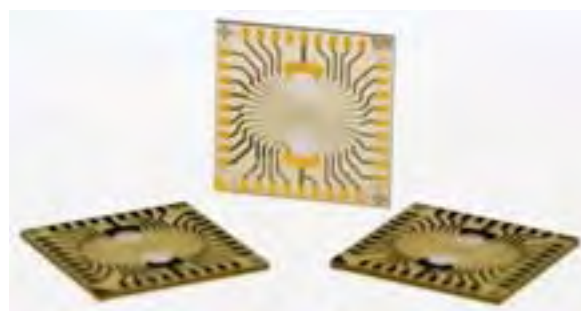
Fig. 2. Glass sensor chip without culture vessel
