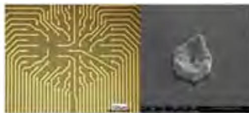
Fig. 1. Left: A 61-electrode microelectrode array on a flexible polyimide substrate. Right: A scanning electron micrograph of a platinised microelectrode.
