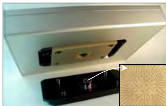
Fig. 2. Open MOGS. Zoom: MEA on glass chip.
