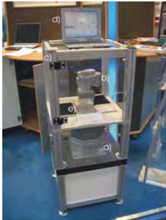
Fig. 4. Automated screening setup with a) Till Photonics „iMIC“ microscope, b) liquid handling robot, c) climate control chamber, d) control computer, and e) multi-well sensor plate
