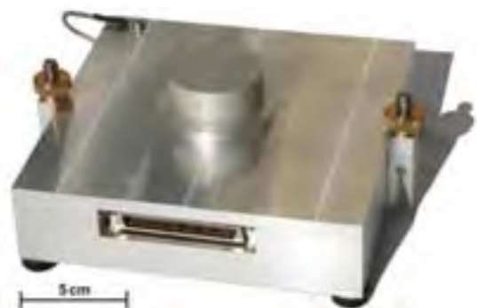
Fig. 2. Test system with 16 electrode channels
