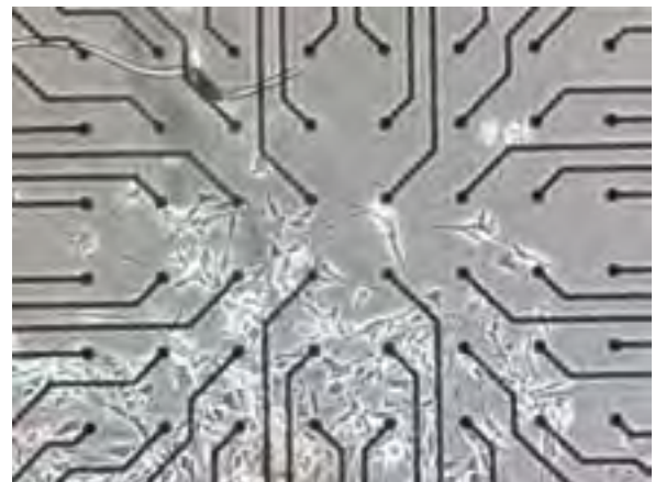
Fig. 3. Image of a MEA plate without coating at day 7. The SH-SY5Y cells are unevenly distributed.
