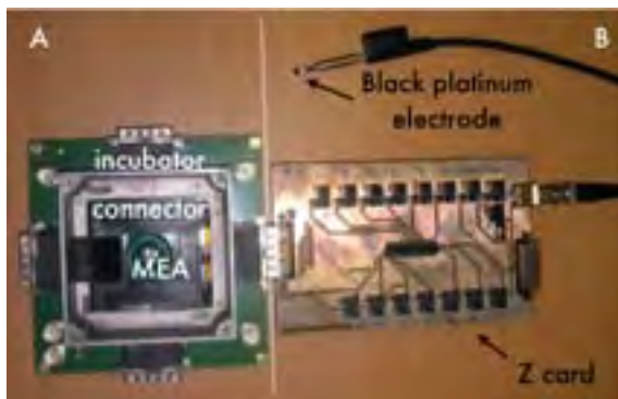
Fig. 1. Set-up for automated impedance spectroscopy. Part A is common with the experiment dedicated to neuronal signal recording while part B is the specific impedance electronic card ("Z card") developed for this study. Switches corresponding to each electrode (13 per card, 8 available positions) are seen.
