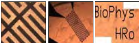
Fig. 4. Primary cortex cells overgrowing different chip structures (IDES, temperature sensor, logo).
