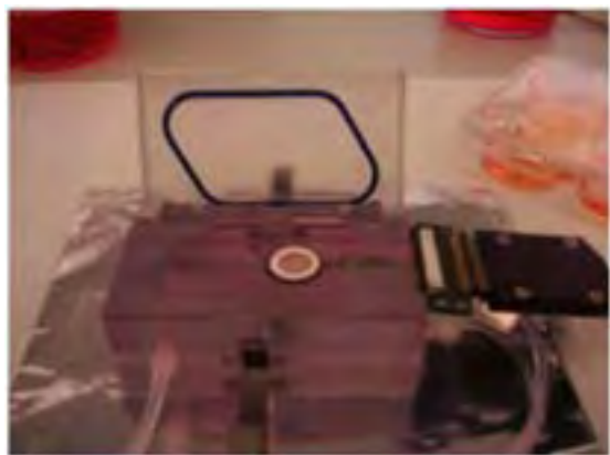
Fig. 2. The recording system inside the incubator
