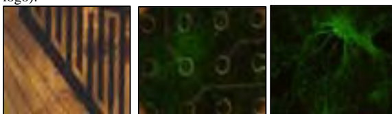
Fig. 5. Stem cell derived neurons cells overgrowing the chip surface. Left: IDES. Center: MEA electrodes. Right: Si3N4-surface.
