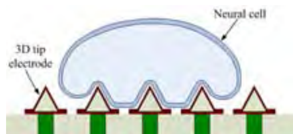
Fig. 1. Conceptual cross-section of a neural cell lying on the tips of a three-dimensional MEA with the attached membrane adapting to the surface topology.
